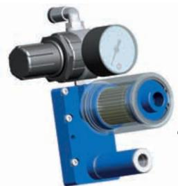
The assembly of a pressure adjuster equipped with pressure gauge and of an FCL filtre on the suction inlet connection of a vacuum generator of the M .. SSX range has allowed creating these small pneumatic suction pumps. Their main features include reduced overall dimensions compared to their technical performance.
